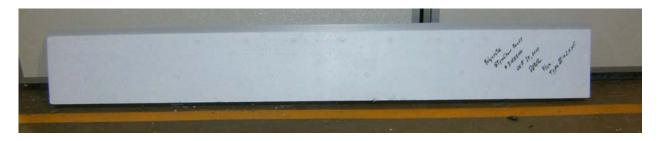
Photograph No. 1: Showing a typical Polycrete flex 850 Insulating Concrete Forms wall panel sample
