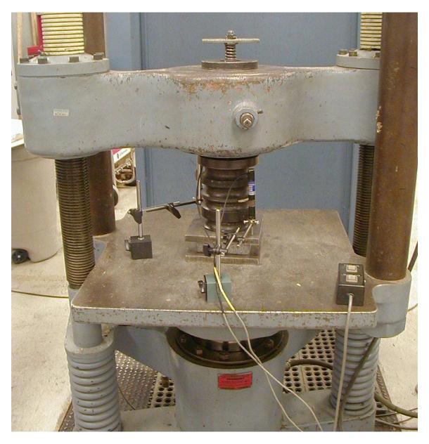
Photograph No. 3: Showing the test setup for compressive resistance.
