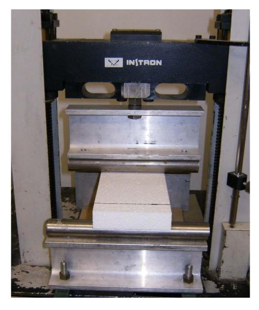
Photograph No. 4: Showing test setup for flexural strength
